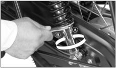
Rear shock absorber adjustment can be made according to the load/road conditions.
