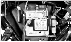
(1) Battery (2) Upper level mark (3) Lower level mark (4) Bolt (5) Bracket
